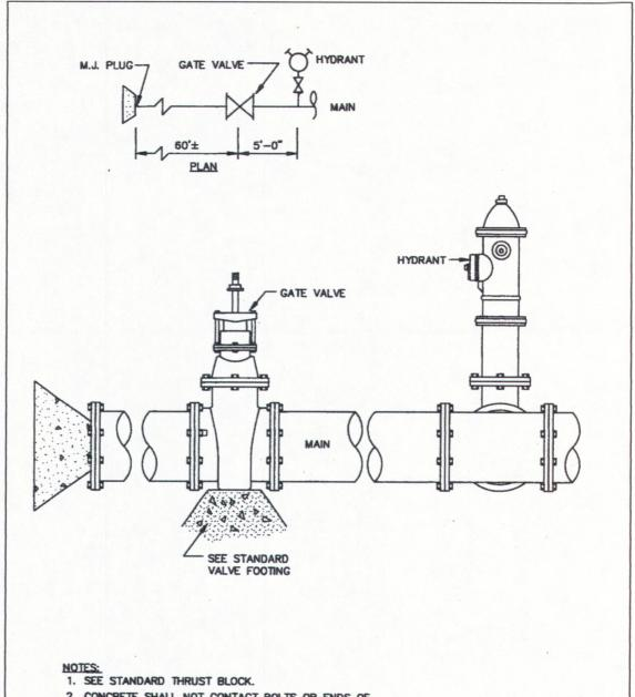
CONCRETE SHALL NOT CONTACT BOLTS OR ENDS OF MECHANICAL FITTINGS.
